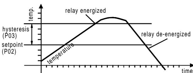
2= Freezing. The compressor resp. the valve is controlled by the N/C contact of K1.
